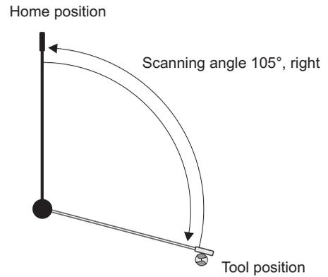
NOTE: Set the maximum angle on the controller equal or larger than the scanning angle. The teach-angle area equals the selected angle plus approximately 5°.
