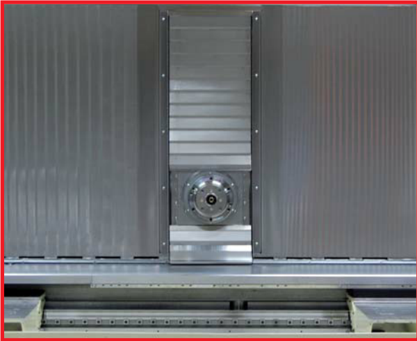
Application of lamella bellows
